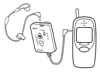
Diagram C. Set-up of MHA100
